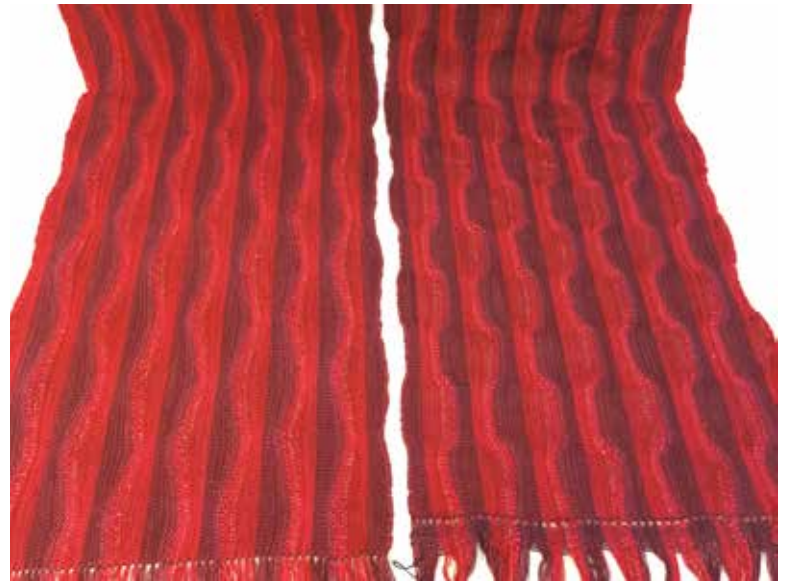
Figure 8. Experiments varying the number of picks between each adjustment of reed position ( left ) and shifting reed position from top to bottom without using the middle positions of the reed ( right )
