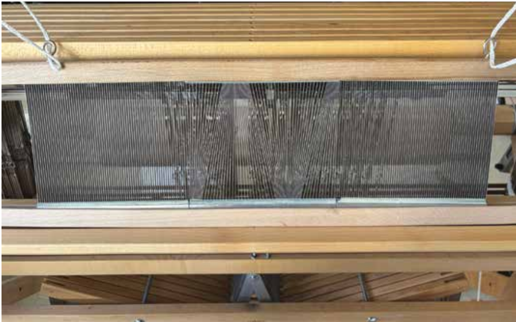
Figure 8. Entering a new phase in my ondulé explorations. Note the sections of plain and fan reed held together in the wooden frame. These sections can be moved around for different projects
