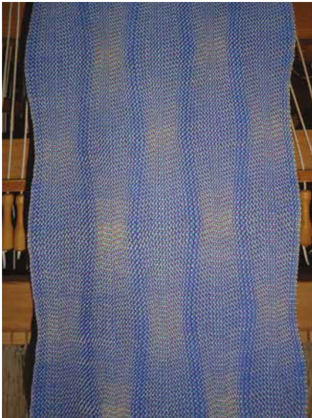
Figure 3a. A shift in warp density at the edges of each fan creates dark lines outlining the fan reed undulations
