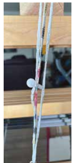
Figure 1b. Color codes on the Texsolv hanging cord help in reed positioning
