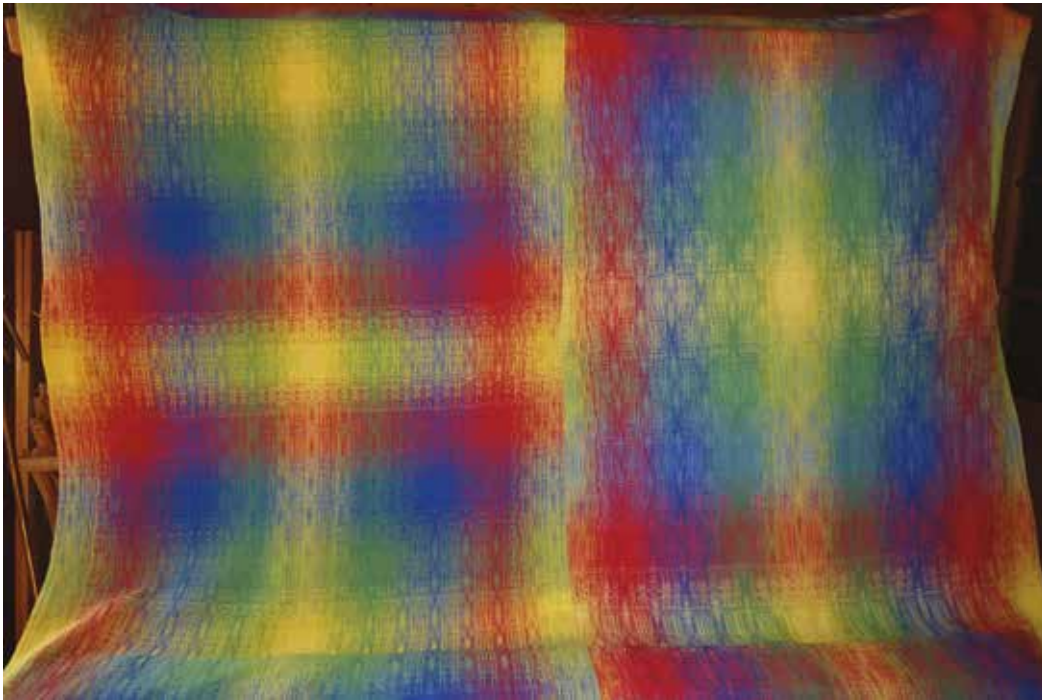
Figure 5c. Color experiment with the fan reed. The piece on the left was woven with the fan reed in its neutral position throughout. For the piece on the right, the reed was repositioned in the manner shown in Figure 5b
