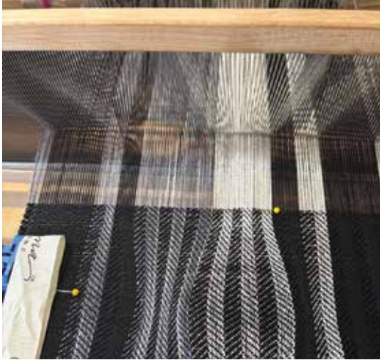
Figure 10. Plain-Fan-Plain twill on the loom. Note the arrangement of the plain and fan sections
