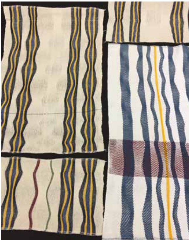
Figure 2. First tests of the fan reed on an Ashford table loom (samples with cream background): interesting, but difficult to control
