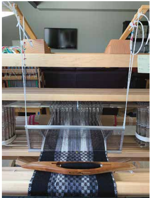
Figure 1a. Project 1 on the loom, weaver's view. Note the wooden add-ons to carry the Texsolv hanging cords
