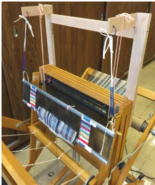
Figure 4. Fan reed modifications on a Wolf Pup loom: added struts hold the reed suspended on elastic bands
