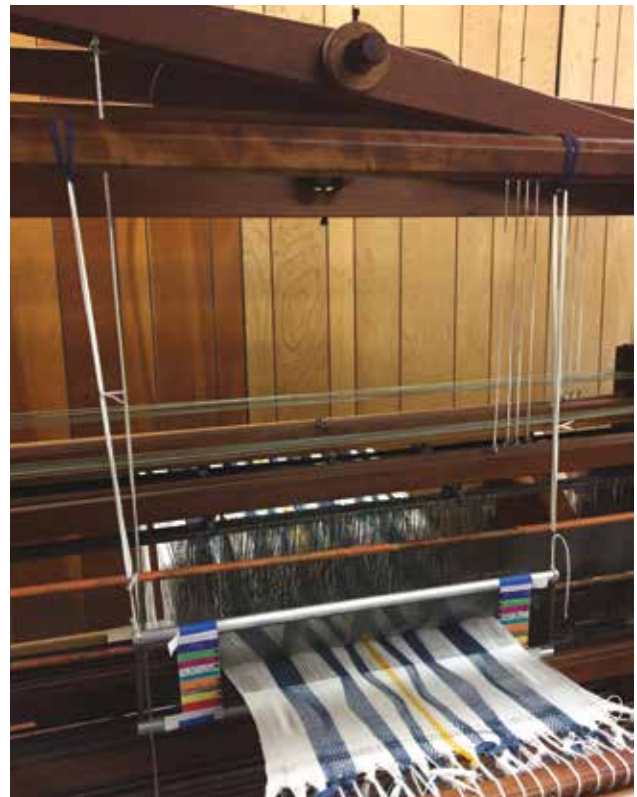
Figure 3. Using the fan reed on a Barbara V countermark loom. Note the suspended reed and colored guide marks at each side of the reed
