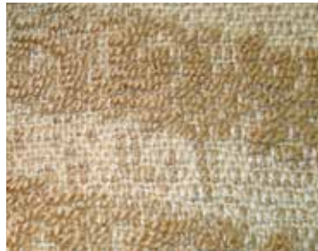
Blouse. Warp and tabby weft are 35/2 tussah silk; pattern weft is 15/2 muga silk. Tied weave, with ties on 12 shafts and pattern on 20 shafts. Ties for blouse closure are in ply-split braiding.
