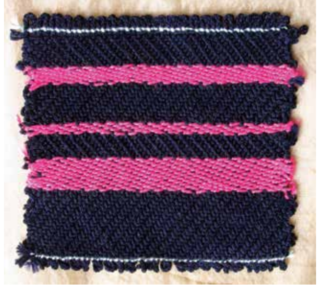
A four-inch sample with twined headers, combining twill and satin structures
