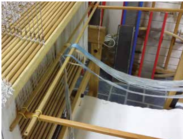
Figure 7. Lease sticks resting behind heddles on the support sticks
