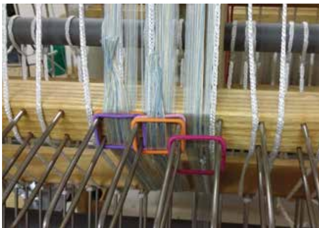
Figure 2. Three sections beamed and secured in place
